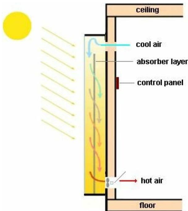
To mount the collector you just have to drill two simple holes in the sunside wall. Inside you see just two holes covered with registers: behind the upper one there is a fan extracting the air from the room and giving it back through the lower hole.
