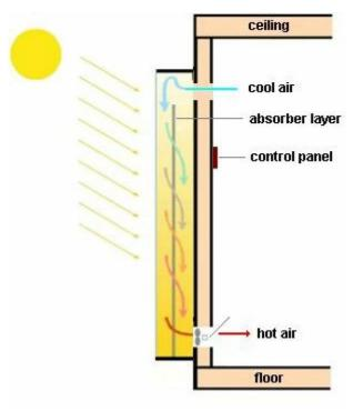
To mount the collector you just have to drill two simple holes in the sunside wall. Inside you see just two holes covered with
